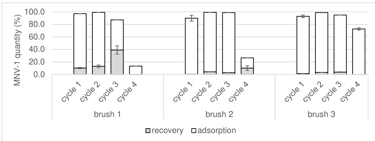
342 Figure 9. PAC coated brush (PAC-B) reusability during four adsorption/desorption cycles. Error
