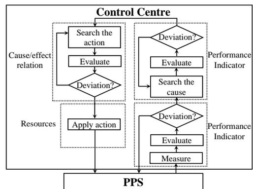
Figure 1: Main steps of the CC control process
